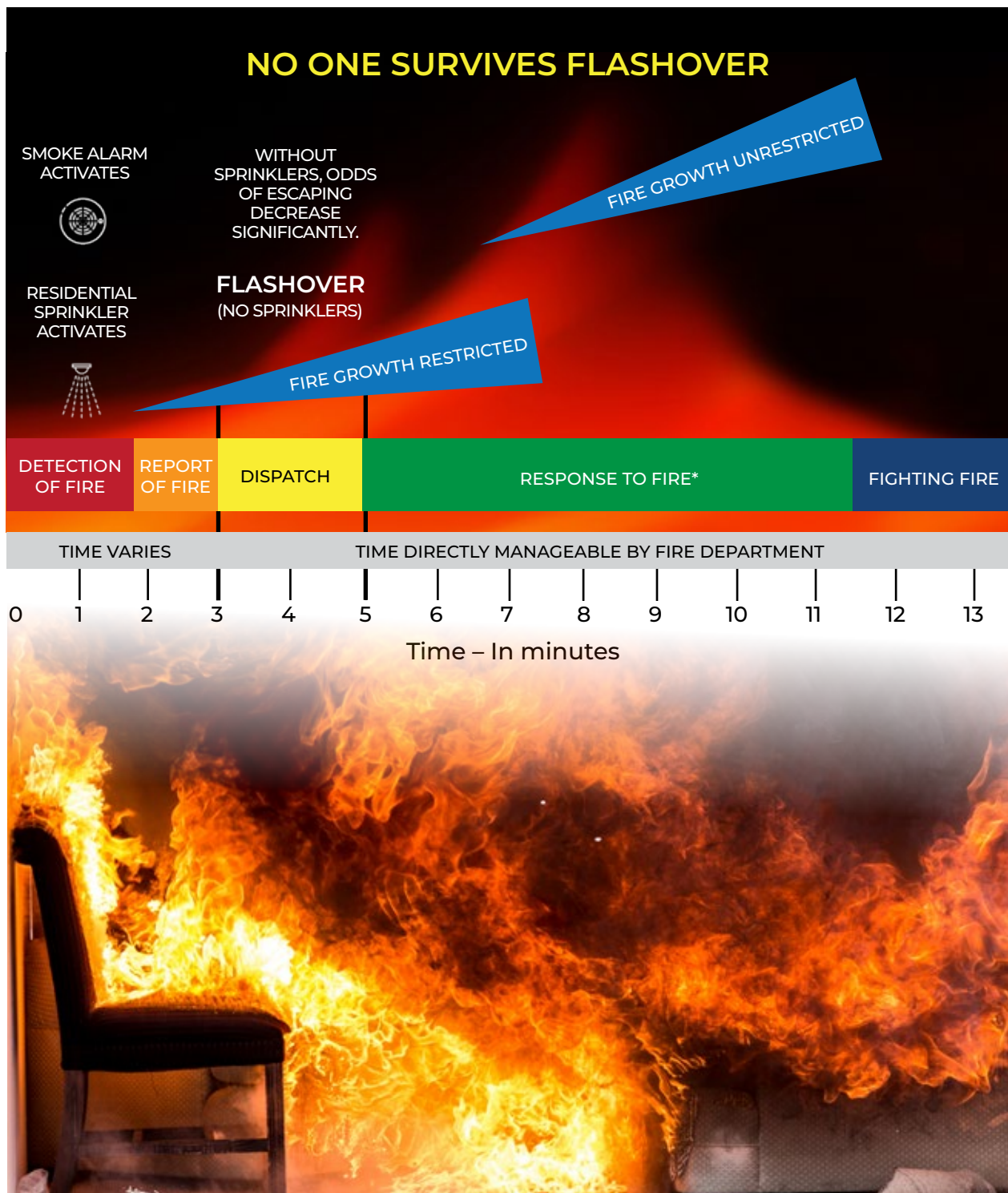
Figure 3.15 Fire Progression to Flashover
