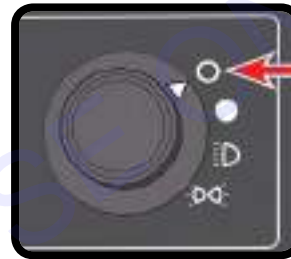
Power Switch Off
