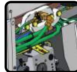
High Voltage Interlock Loop Yellow Wire
