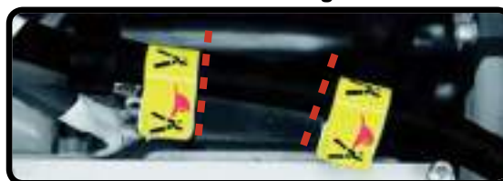
Cut 12V Battery Positive Cable As Marked
