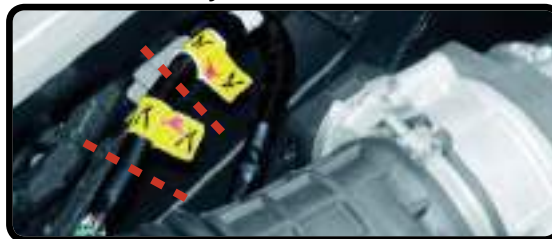
Cut 12V Battery Negative Cable As Marked
